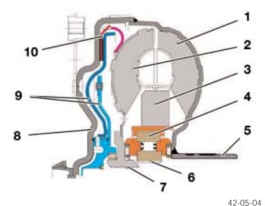
Torque Converter & Lockup Clutch
